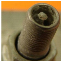
Heavily corroded sensor
